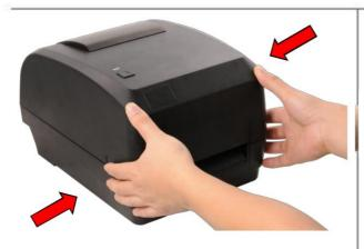
Open the printer top cover by pressing the top cover open tabs located on each side of the printer.
