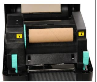
3. Insert the left side of ribbon rewind spindle to the ribbon rewind hub first then insert the right side of ribbon rewind spindle to the hole at the right side of ribbon mechanism.
