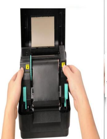
8. Turn the ribbon rewind hub until the ribbon plastic leader is thoroughly wound and the black section of the ribbon covers the print head.
