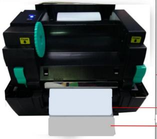
6. Press the FEED button to test.
