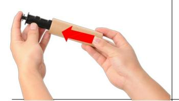
2. Insert the paper core to the ribbon rewind spindle.
