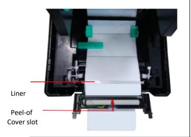
Open the peel-off cover. Feed the liner into peel-off cover slot.
