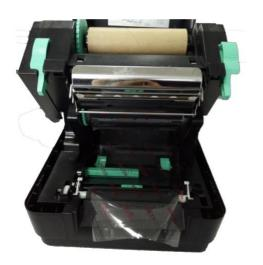
6. Insert the left side of ribbon supply spindle to the ribbon supply hub first then insert the right side of ribbon supply spindle to the hole at the right side of ribbon mechanism.
