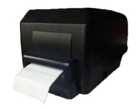
Close the print head mechanism and printer cover. Use the DiagTool to set the printer for cutter mode by selecing "CUTTER" option for Post-Print Action setting then click "Set" button to enable the cutter mode.
