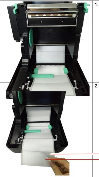
Refer to chapter 3.3.1 to install the label. Use "Diagnostic Tool" to set the media sensor type and calibrate the selected sensor.
