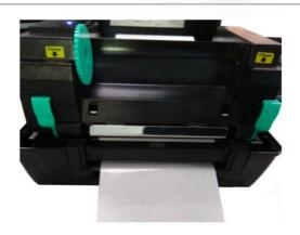
5. Close the print head mechanism and printer cover. Printer is ready for peel-off mode.
