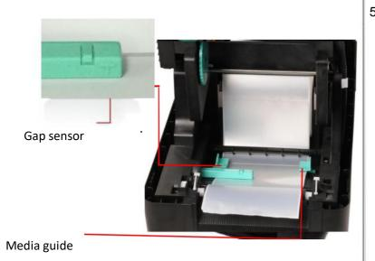
i. Feed the paper, printing side face up, through the media bar, media sensor and place the label leading edge onto the platen roller. Move the media guides to fit the label width.
