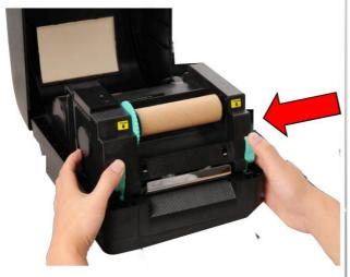
4. Push the print head release button to open the print head mechanism.
