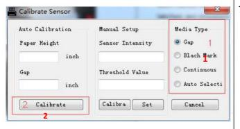
Use "Diagnostic Tool" to set the media sensor type and calibrate the selected sensor. (Start the "Diagnostic tool" → Select the "Printer Configuration" tab → Click the "Calibrate Sensor" button )
