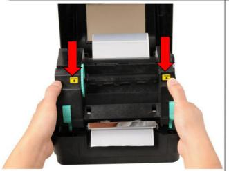
Close the print head mechanism by both hands and make sure the latches are engaged securely.
