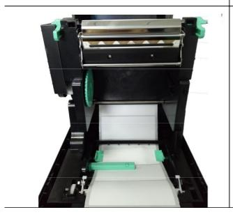
5. Refer to chapter 3.3.1 to install the label. Use "Diagnostic Tool" to set the media sensor type and calibrate the selected sensor.
