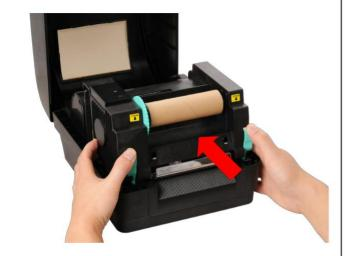
4. Push the print head release button to open the print head mechanism.
